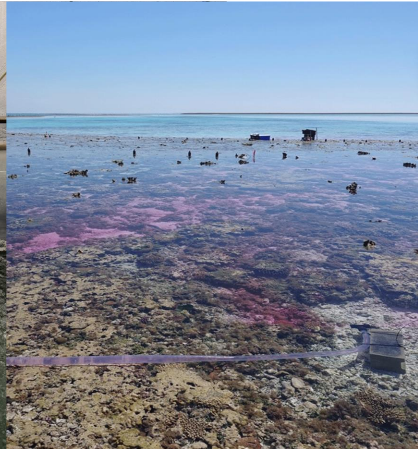
Dye plumes as part of an OAE experiment in an Australian coral reef flat study site. SOURCE: Cyronak et al. OAE Guide 2023 Ch 7
