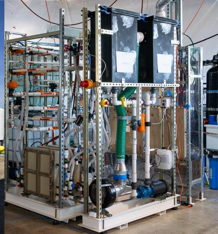
Ebb Carbon's electrochemical OAE system. SOURCE: https://www.eisamanlab.com/ebb-carbon
