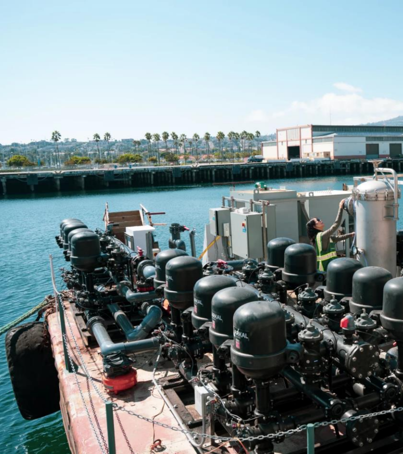
Captura's direct ocean capture system. SOURCE: https://capturacorp.com/technology/
